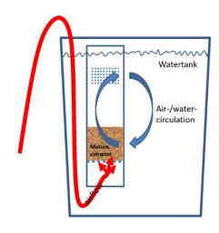
If no power or air blower is available, the materials can be put in the 200 liter tank and stirred manually for minimum 1 hour. Stirring it manually is less effective but better than not doing it.
